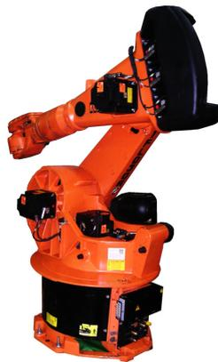
**Figura 1.3: Robot KUKA KR150.**
