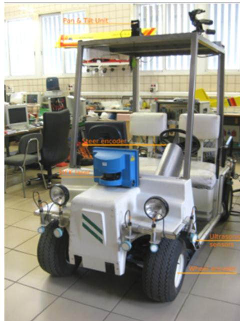
Figura 2.5: Robot Romeo-4R. Sensores (II).
